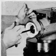
Figure 21A Grinding Wheel Collet Assemblies are Quickly Interchanged by Removing Socket Head Screw
